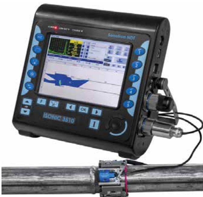
Phased Array set on small bore pipe
